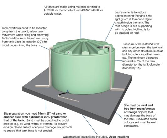
ball valve please ensure flexible pipe is connected to ball valve to allow room for movement and, which will ensure that the tank is not damaged. Ensure that pipe work is well clear of moving vehicles ensuring no damage to tank or fittings. An inline filter must be installed between the tank and the pump to protect appliances connected to pump delivery.
